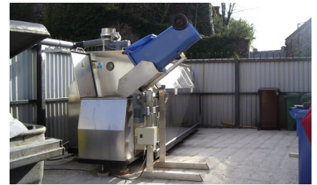
The bin lift makes it easier to handle large volumes of food waste. Talbot Hotel in Wexford, Ireland has a bin lift for their model T240.
