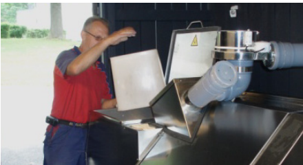
The food waste is fed in to the machine's front end. It is convenient to be able to treat the food waste daily. Picture from Gamleby Folk Highschool, Sweden.
